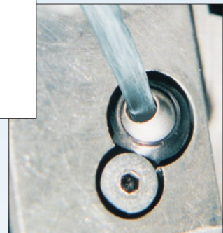
BlackEye installed on quick change turning tool.
